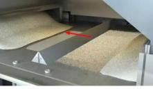
Deposition of a layer of powder
