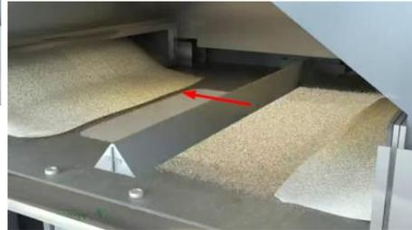
Deposition of a layer of powder
