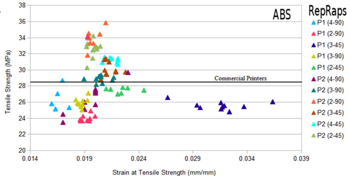
Mechanical Properties of components Fabricated with Open-Source 3-D Printers
