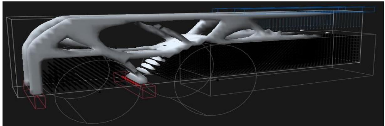
Material distribution in the width of the part - TopoStruc
